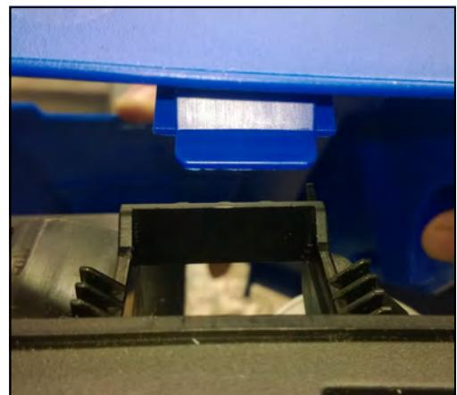
**Disassembly / assembly of pump cover.**
