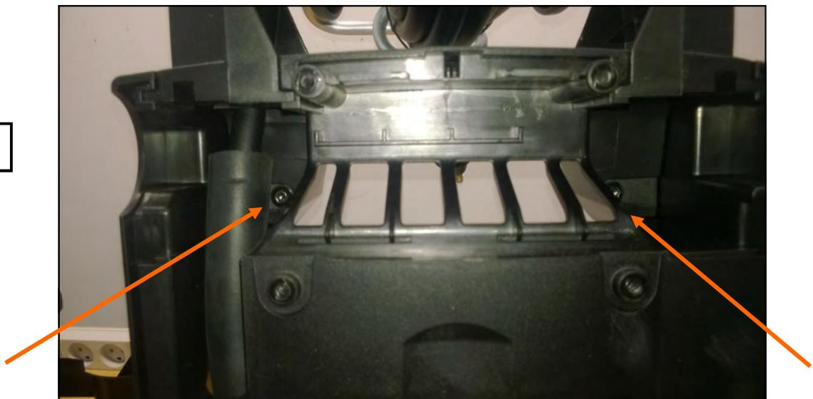
**Disassembly / assembly of the high pressure hose - X-TRA models.**
